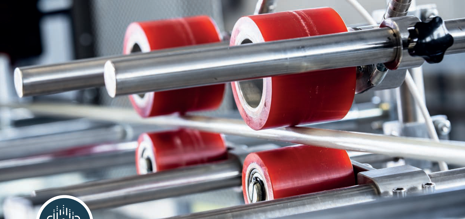
Rollers for measuring the haul-off speed.
