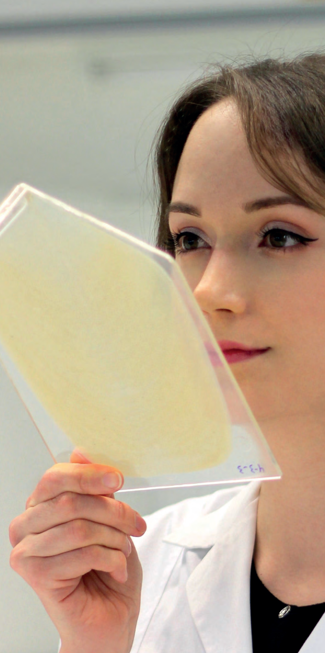
Sandwich test specimen with recycled core (brown) and a skin material without odor-reducing additives during sensory evaluation.
