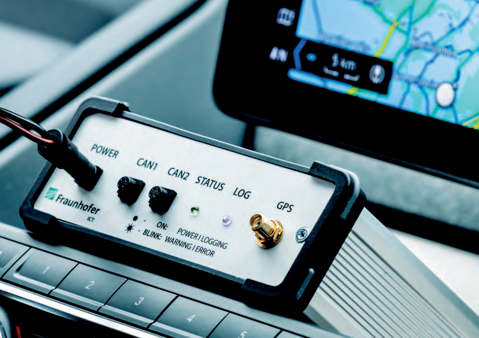
Data logger for autonomous recording of a wide variety of measurement data in cars, trucks or production plants.
