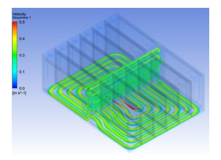
CFD simulation - calculation of the flow velocity in the cooling system of a battery module
