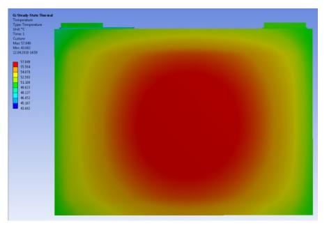
Thermal simulation model of a 60 Ah BEV cell at 4 C charge rate
